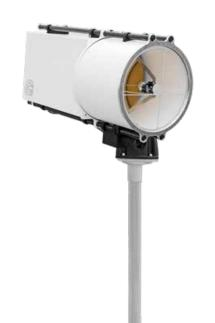
$\rightarrow$  The **scanfeld** remote monitoring system takes a new approach. The airspace of the entire plant is scanned by the FTIR spectrometer, the chemical composition of the air is spectroscopically analysed and the gas is identified. Three software modules control the system, visualise and track gas clouds, mark hazard areas and issue an alarm in accordance with the threat level.
